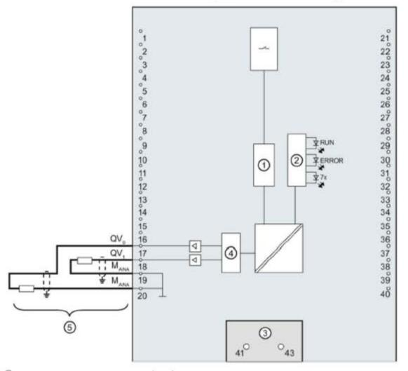
Wiring: Voltage output
