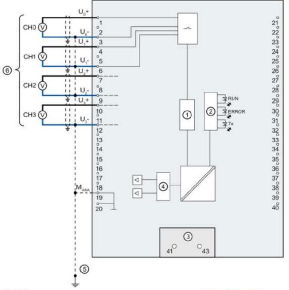
Wiring: Voltage measurement
