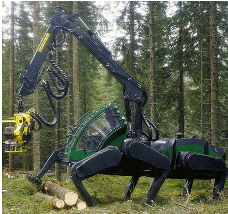
The Plusjack Walking Harvester Full-Scale Prototype (Ismoilov, 2016)
